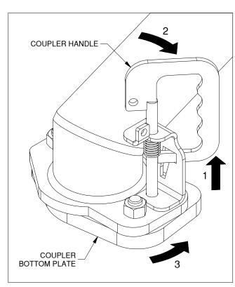
Figure B1: Coupler in "open" position
