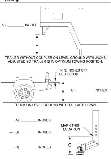
Figure A5: Coupler height determination.
