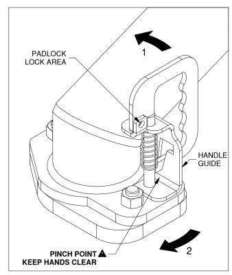
Figure B2: Coupler in "closed" position
